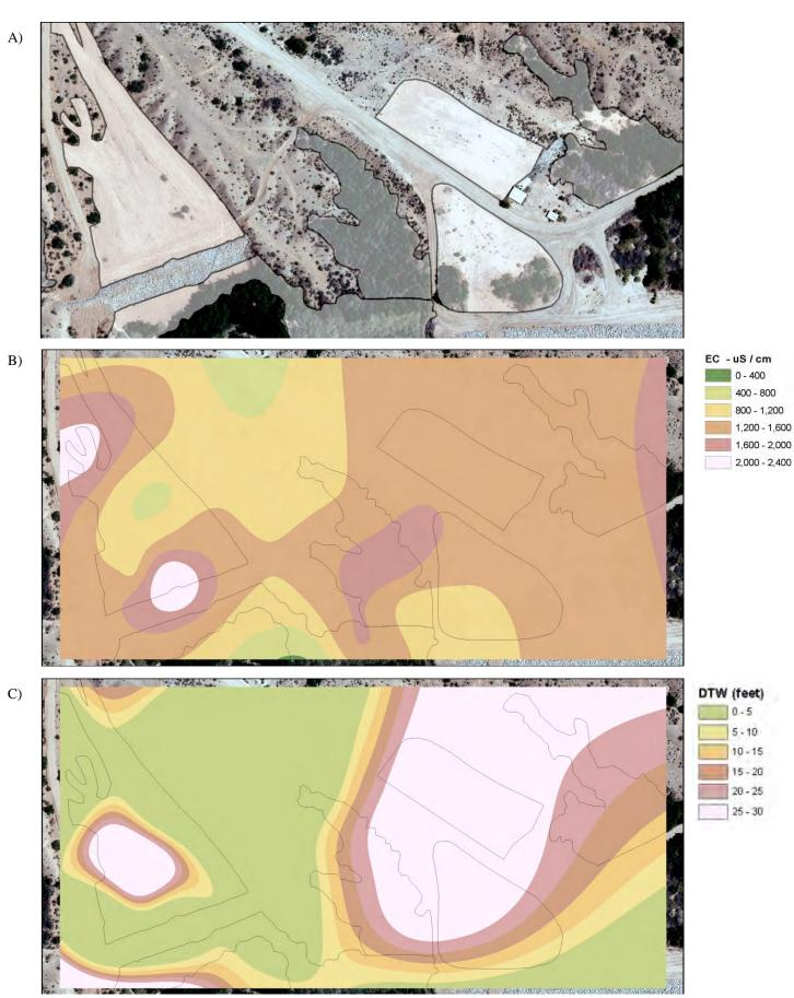
Figure 3: Soil analysis areas within the Cottonwood Cell North planting area: (A) outlined areas, (B) electrical conductivity, and (C) depth to water.
