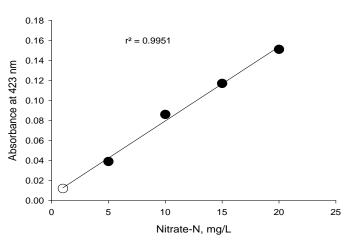
Figure 2. Calibration curve for nitrate-N assay.
