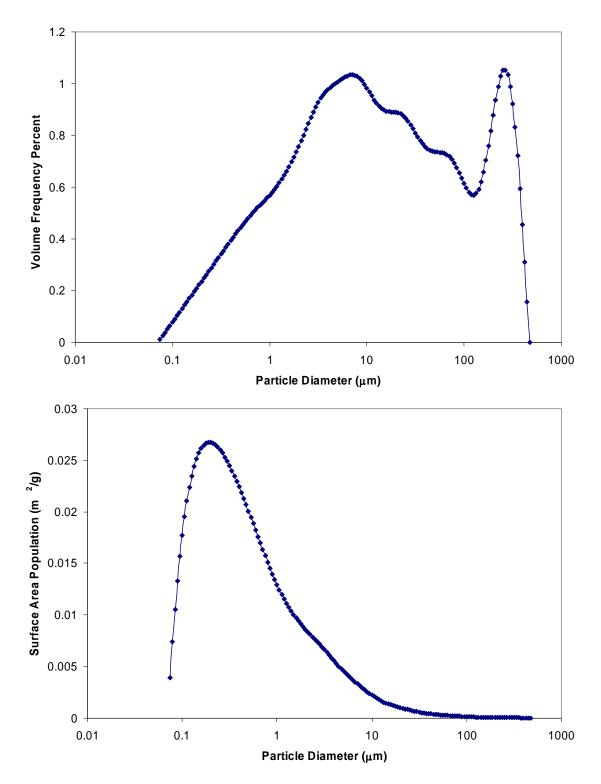
Figure 5. (a) Particle volume frequency vs. diameter and (b) particle surface area population vs. diameter for the Nature Preserve sample.
