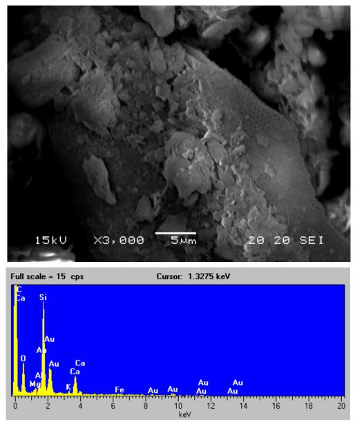
Figure 8. Scanning electron micrograph and EDX spectrum of the Las Vegas Bay sample (magnification 3,000x). Spectrum composition consistent with the presence of quartz and calcite in this sample.
