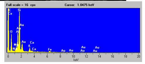
Figure C-15. Scanning electron micrograph, EDX spectrum, and elemental composition of the third particle of the Las Vegas Wash 0.8 mile sample (magnification 2,000x).
