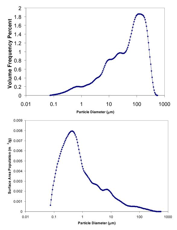
Figure 4. (a) Particle volume frequency vs. diameter and (b) particle surface area population vs. diameter for the Duck Creek sample.
