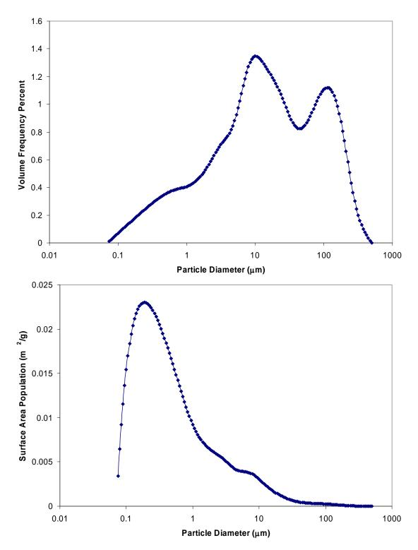
Figure 3. (a) Particle volume frequency vs. diameter and (b) particle surface area population vs. diameter for the Las Vegas Wash 10.75 mile sample.
