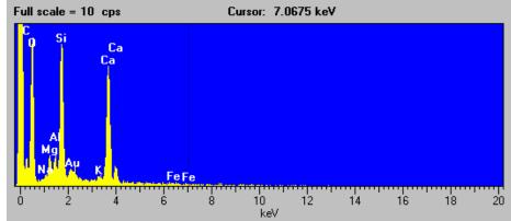
Figure C-26. Scanning electron micrograph, EDX spectrum, and elemental composition of the fourth particle of the Las Vegas Wash 10.75 mile sample (magnification 900x).
