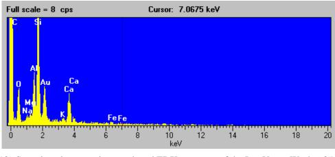
Figure 13. Scanning electron micrograph and EDX spectrum of the Las Vegas Wash 6.05 mile sample (magnification 600x). Spectrum consistent with the presence of plagioclase in this sample.
