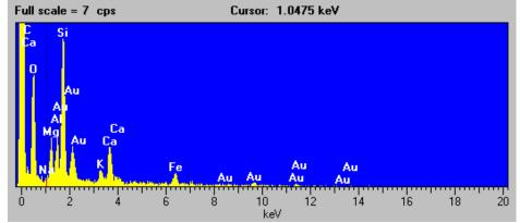
Figure C-37. Scanning electron micrograph, EDX spectrum, and elemental composition of the fourth particle of the Nature Preserve sample (magnification 2,700x).
