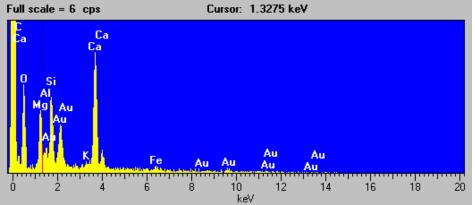
Figure C-3. Scanning electron micrograph, EDX spectrum, and elemental composition of the second particle of the Las Vegas Bay sample (magnification 3,300x).
