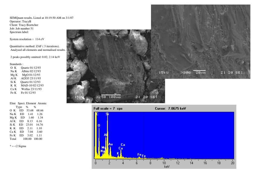
Figure C-8. Scanning electron micrograph, EDX spectrum, and elemental composition of the first particle of the Las Vegas Bay duplicate sample (magnifications 250x and 800x).
