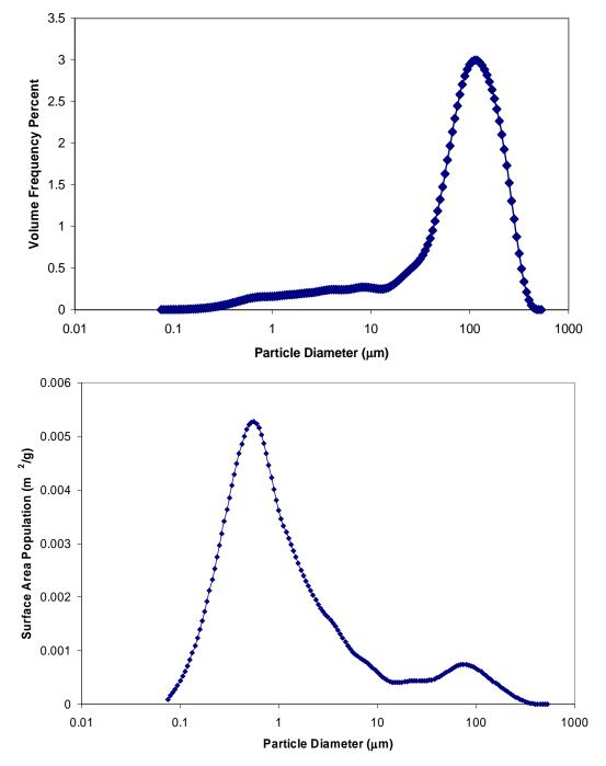
Figure 2. (a) Particle volume frequency vs. diameter and (b) particle surface area population vs. diameter for the Las Vegas Bay sample.
