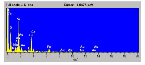
Figure C-5. Scanning electron micrograph, EDX spectrum, and elemental composition of the fourth particle of the Las Vegas Bay sample (magnification 850x).
