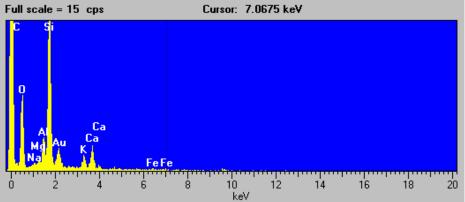
Figure C-30. Scanning electron micrograph, EDX spectrum, and elemental composition of the third particle of the Duck Creek sample (magnification 1,600x).
