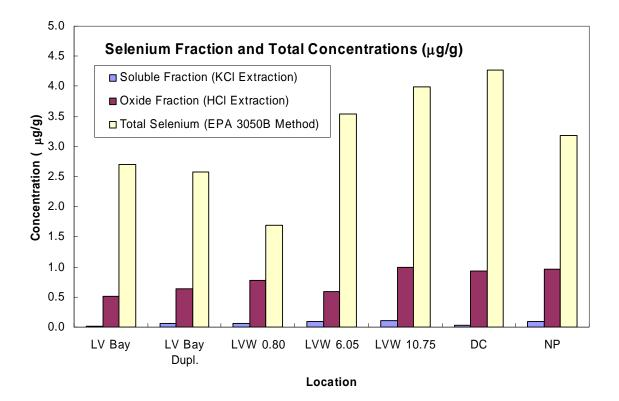
Figure 16. Concentrations of soluble selenium, selenium associated with oxides, and total selenium  $(\mu g/g)$ .
