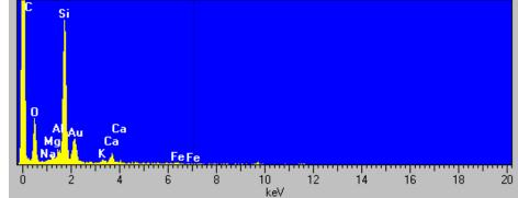
Figure C-9. Scanning electron micrograph, EDX spectrum, and elemental composition of the second particle of the Las Vegas Bay duplicate sample (magnification 1,100x).
