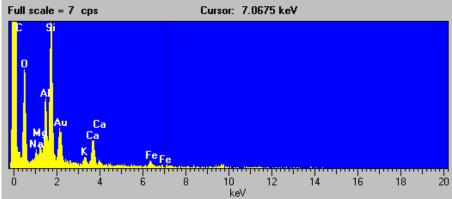
Figure 9. Scanning electron micrograph and EDX spectrum of the Las Vegas Bay duplicate sample (magnifications 250x and 800x). Spectrum consistent with the presence of biotite in this sample.
