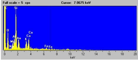
Figure C-21. Scanning electron micrograph, EDX spectrum, and elemental composition of the fourth particle of the Las Vegas Wash 6.05 mile sample (magnification 3,500x).
