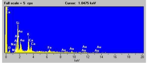
Figure C-35. Scanning electron micrograph, EDX spectrum, and elemental composition of the second particle of the Nature Preserve sample (magnification 4,300x).
