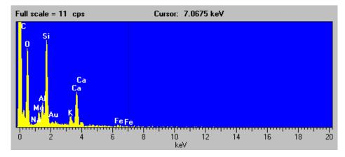
Figure C-23. Scanning electron micrograph, EDX spectrum, and elemental composition of the first particle of the Las Vegas Wash 10.75 mile sample (magnification 2,000x).
