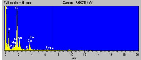
Figure C-10. Scanning electron micrograph, EDX spectrum, and elemental composition of the third particle of the Las Vegas Bay duplicate sample (magnification 1,100x).
