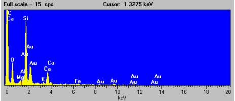
Figure C-4. Scanning electron micrograph, EDX spectrum, and elemental composition of the third particle of the Las Vegas Bay sample (magnification 3,000x).
