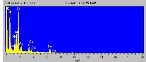
Figure C-19. Scanning electron micrograph, EDX spectrum, and elemental composition of the second particle of the Las Vegas Wash 6.05 mile sample (magnification 2,500x).
