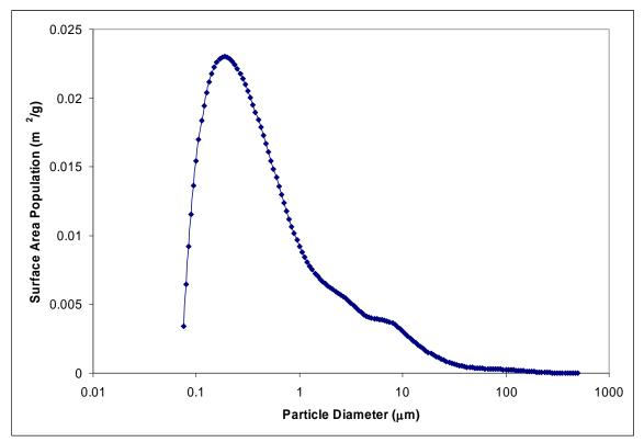
Figure A-5. (a) Particle volume frequency vs. diameter and (b) particle surface area population vs. diameter for the Las Vegas Wash 10.75 mile sample.
