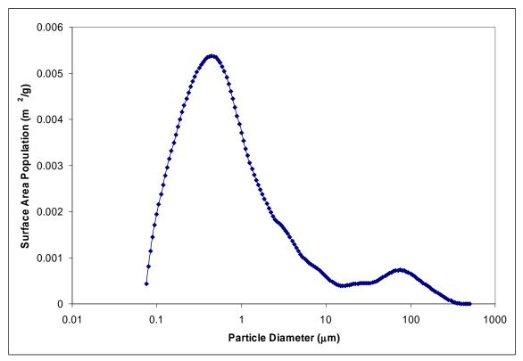
Figure A-2. (a) Particle volume frequency vs. diameter and (b) particle surface area population vs. diameter for the Las Vegas Bay duplicate sample.
