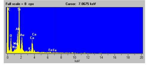
Figure C-20. Scanning electron micrograph, EDX spectrum, and elemental composition of the third particle of the Las Vegas Wash 6.05 mile sample (magnification 600x).
