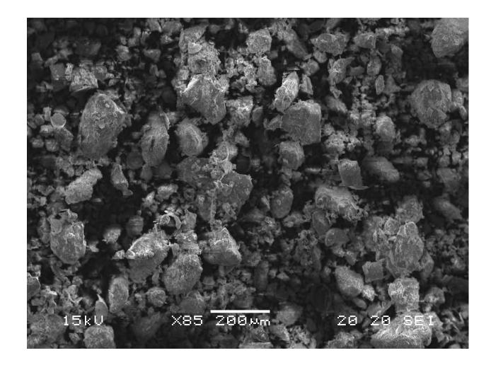
Figure C-12. General view of the Las Vegas Wash 0.8 mile sample. Magnification 85x.
