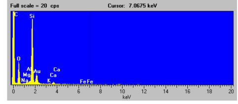
Figure C-11. Scanning electron micrograph, EDX spectrum, and elemental composition of the fourth particle of the Las Vegas Bay duplicate sample (magnification 1,100x).
