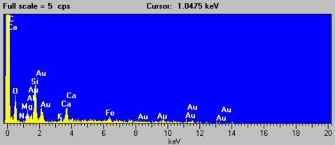
Figure C-6. Scanning electron micrograph, EDX spectrum, and elemental composition of the fifth particle of the Las Vegas Bay sample (magnification 1,400x).
