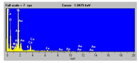
Figure C-13. Scanning electron micrograph, EDX spectrum, and elemental composition of the first particle of the Las Vegas Wash 0.8 mile sample (magnification 650x).
