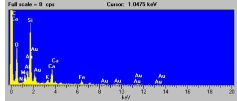
Figure C-14. Scanning electron micrograph, EDX spectrum, and elemental composition of the second particle of the Las Vegas Wash 0.8 mile sample (magnification 400x).
