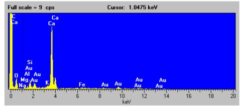
Figure 12. Scanning electron micrograph and EDX spectrum of the Las Vegas Wash 0.8 mile sample (magnifications 600x and 1,200). Spectrum consistent with the presence of calcite in this sample.
