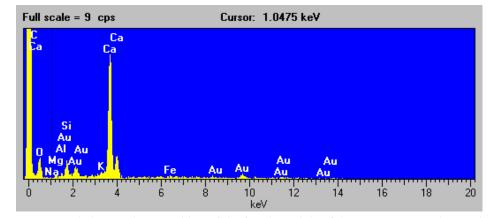
Figure C-16. Scanning electron micrograph, EDX spectrum, and elemental composition of the fourth particle of the Las Vegas Wash 0.8 mile sample (magnifications 600x and 1,200).
