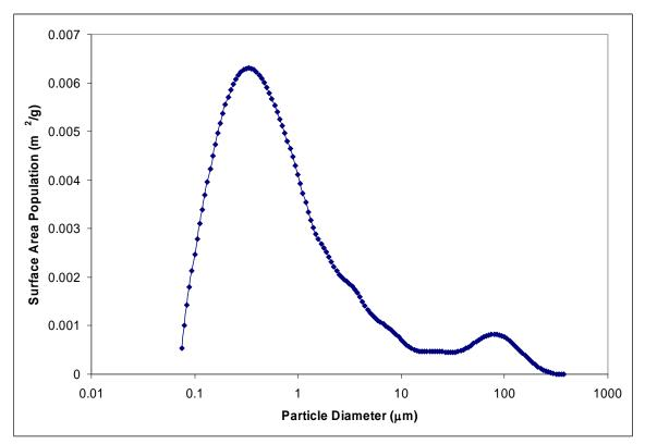
Figure A-3. (a) Particle volume frequency vs. diameter and (b) particle surface area population vs. diameter for the Las Vegas Wash 0.8 mile sample.
