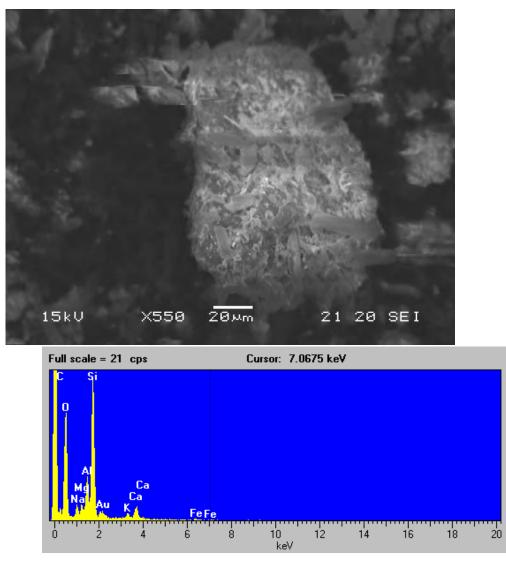
Figure C-25. Scanning electron micrograph, EDX spectrum, and elemental composition of the third particle of the Las Vegas Wash 10.75 mile sample (magnification 550x).
