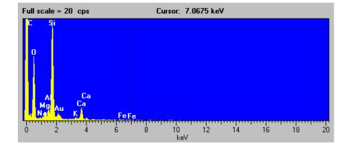
Figure C-24. Scanning electron micrograph, EDX spectrum, and elemental composition of the second particle of the Las Vegas Wash 10.75 mile sample (magnifications 600x and 1,000x).
