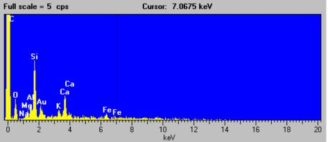
Figure C-29. Scanning electron micrograph, EDX spectrum, and elemental composition of the second particle of the Duck Creek sample (magnification 2,500x).
