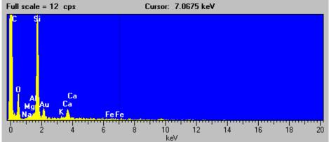
Figure C-32. Scanning electron micrograph, EDX spectrum, and elemental composition of the fifth particle of the Duck Creek sample (magnification 2,300x).
