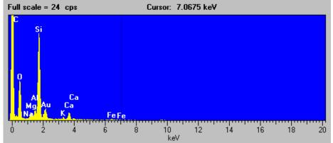
Figure C-18. Scanning electron micrograph, EDX spectrum, and elemental composition of the first particle of the Las Vegas Wash 6.05 mile sample (magnification 1,200x).
