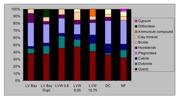
Figure 6. Semiquantitative mineralogical composition of sediment samples.
