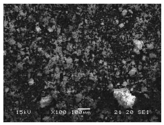
Figure 14. General view of the Las Vegas Wash 10.75 mile sample. Magnification 100x.
