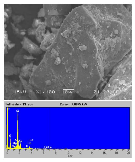
Figure 10. Scanning electron micrograph and EDX spectrum of the Las Vegas Bay duplicate sample (magnification 1,100x). Spectrum consistent with the presence of mostly quartz and some orthoclase in this sample.
