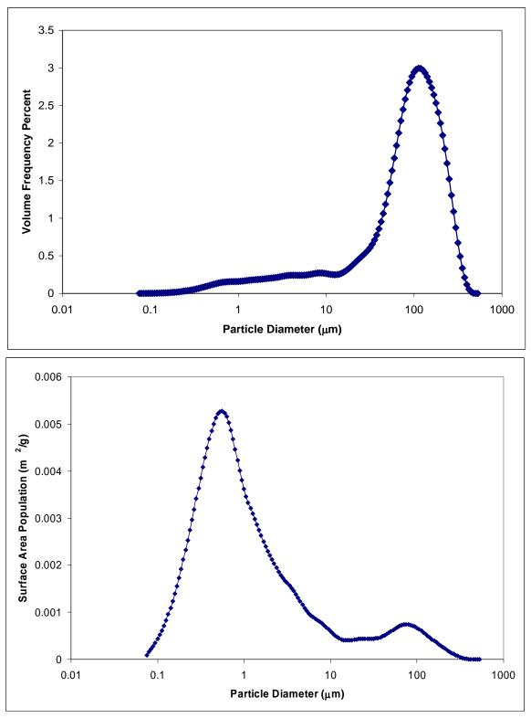
Figure A-1. (a) Particle volume frequency vs. diameter and (b) particle surface area population vs. diameter for the Las Vegas Bay sample.
