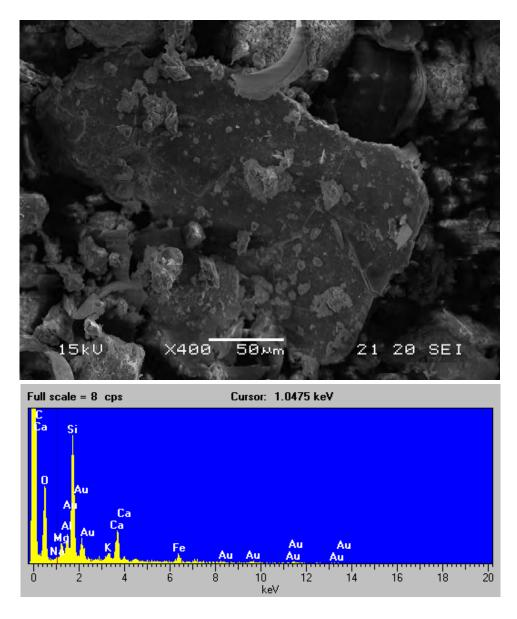
Figure 11. Scanning electron micrograph and EDX spectrum of the Las Vegas Wash 0.8 mile sample (magnification 400x). Spectrum consistent with the presence of mostly quartz, calcite, and dolomite in this sample.
