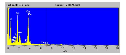
Figure C-28. Scanning electron micrograph, EDX spectrum, and elemental composition of the first particle of the Duck Creek sample (magnifications 3,000x and 5,000x).
