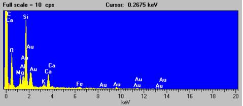
Figure C-2. Scanning electron micrograph, EDX spectrum, and elemental composition of the first particle of the Las Vegas Bay sample (magnification 1,400x).
